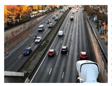
Wintics Cityvision software installed at Neuilly analyses video stream from 5 Hikvision thermal cameras. Cityvision uses Al to measure, analyze and visualize traffic data from the boulevard to assist in measuring the state and type of traffic as well as how and when people use the 10 traffic lanes. Once the project is complete, the installation will also assist the city in monitoring traffic to measure its positive impact and changes in
