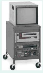
19-1/4" Equipment Cart. An affordable cart for studio or mobile use. Comes complete with two shelves and four removable 19-1/4" (11U) rack rails. Two position bottom shelf can be fixed at center height for compact electronics. Sturdy, strong, heavy-duty steel construction. Charcoal Grey enamel finish. Rolls easily on 3-inch dual-wheel castors. Two locking castors for operating stability. 30"H x 21"W x 26"D (762 x 533 x 660mm). Charcoal Grey. K8706 Shpg. wt. 24.6 kgs.
