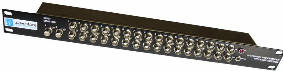
**The Wavestore Passive Access Panel** provides for up to 32 video and up to 16 audio inputs. A 1.2M multi-way cable is included that enables physical access to the server during operation.
