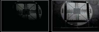
Double Scan CCD With Conventional WDR
