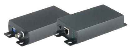
VIP02 IP extender is designed to extend the transmission range of any IP based device up to 1.8 Km over existing coaxial cable. It is completely transparent to protocols, codes, and applications ensuring compatibility with any IP camera and its management software. It is a perfect solution for sending IP video links from remote camera installation utilising existing RG59 coax cable infrastructure up to 1800 meters
