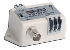
The Vigitron Vi6100VT is an advanced active device that transmits high resolution color or B&W video over unshielded twisted pair wires. The Vi6100VT uses Category 2-7 UTP wire at distances up to 6,000 feet (1830 m) and is designed to be paired with any Vigitron Vi6100 series Active Receivers.
