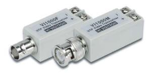
The Vigitron VI1000 and VI1010 are passive video transmission devices that transmit video over unshielded twisted pair wires, point-to-point, for distances up to 1100 feet (330 m). They use Category 2-5 twisted pair wires, are easy to install and cost effective, and do not require power. Their unique and compact design allows mounting directly to the video source or receiver without any additional cabling.
