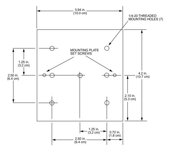
Figure 1 **Mounting Diagram**
