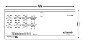
Kollector Elite Server is a rack mount, standalone and network ready video recorder providing extended continuous recording. The front panel features two rack installation handles and a convenient and secure user interface. Behind a key locked door is an array of conveniently located controls including a power switch, a reset switch (for service purposes), 3.5-inch floppy drive and CD-R/W drive and an array of hard drives.
