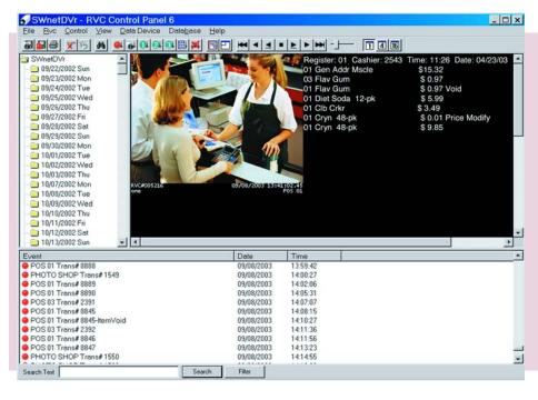
The easy-to-use Control Panel software allows you to connect to a Verint Lanex netDVR via standard phone lines, network, or local access cable. Once connected, you can retrieve video, change settings or search for a specific transaction.
