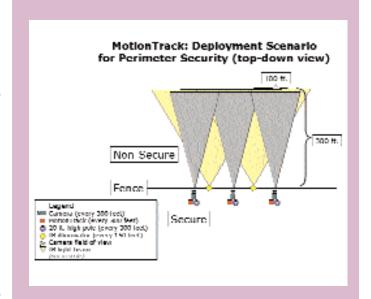
Deploying cameras perpendicular to the fence line provides maximum depth of protection, optimal probability of detection and reduced camera costs
