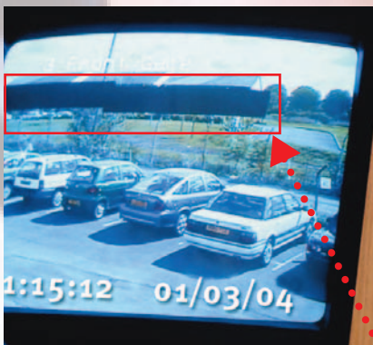
Privacy zones are ideal to secure commercial buildings in areas where private housing is also present.
