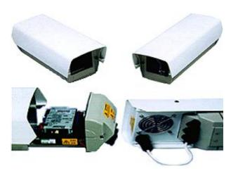
Ease of access for serviceability and installation has been provided with the design of a hinged retained body. The RX range of Super Connoisseur (LONG) incorporates a built-in 10 function AC telemetry receiver (Molynx TRX228) with C type or D type telemetry interface and either 230V or 24V AC operation.
