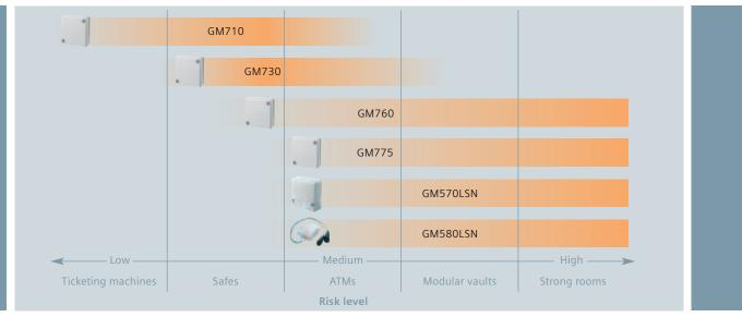
Seismic detectors application range
