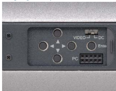
Control buttons for the OSD menu for configuring the comprehensive functions.
