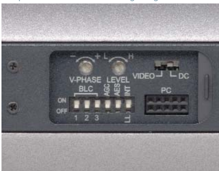
Simple DIP switches for configuring functions.
