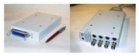
up to 4 PAL/SECAM v/cams - HDD20Gb - RISC processor Hitachi Super H3 - Newest video compression technologies - Simplest setting up of work parameters and access to stored video via standard LPT port of your PC
