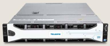
S-VMX NVR is the network video recorder component of the Teleste S-VMX system designed to operate in a multi-host environment. It supports multiple simultaneous user connections to, and multiple concurrent views of recorded material.
