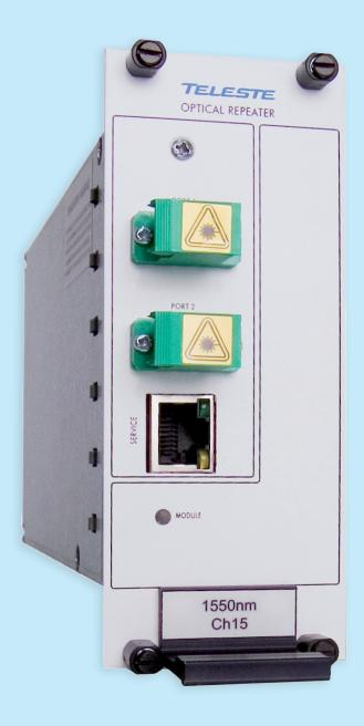
COR repeaters are part of the extensive CFO OPX platform that complies to ITU G.694.2 CWDM grid. These non-regenerative repeaters provide a cost effective way to cover extreme transmission distances over optical fibre. Depending on system up to two or three repeater units can be connected in series to make a line in which each leg have a maximum of 20 dB link budget available.
