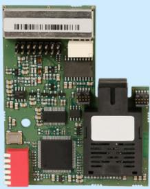
This selected CFO series is capable of proving an optical transmission for a composite video, one serial data and one contact closure type I/O channel. Data and CC communication is 2-way. Data channel is configurable to various RS modes by DIP switches.
