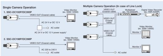
\*An AC 24 V power supply box is needed for the AC 24 V powered models.
