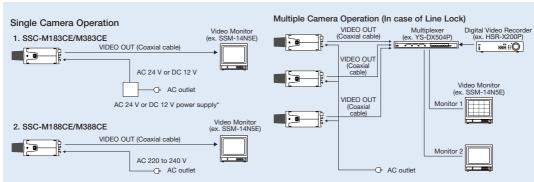
\*An AC 24 V power supply box is needed for the AC 24 V powered models.
