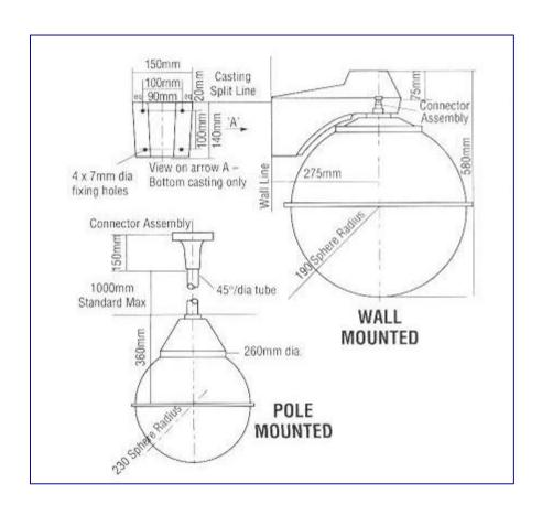
The Marquis range of surveillance domes is designed to satisfy the increasing demand for discreet internal surveillance. Specified most frequently for retail and commercial premises, it is essential that a range of product options are available to meet any combination of technical requirements. Such a choice of options are available from the Marquis range, providing the optimum opportunity to meet all specifications.
