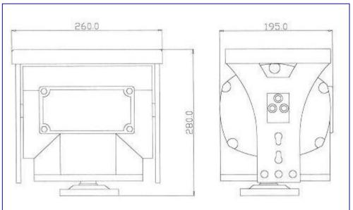
The Shawley Duke PT 461 head is a heavy duty dedicated top mount unit, which is built to support greater pay loads and operate reliably in severe weather environments. IR lamps fit directly to side supports via 'keyhole slots' - a particular advantage when installing in awkward situations.
