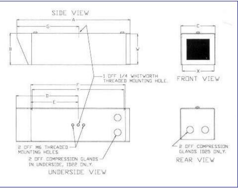
The ID range of camera housings is specifically designed for internal applications only. They provide dust proof enclosures which are ideal for static cameras with fixed focal lengths. The ID22 and ID25 are supplied with an adjustable camera platform, two cable glands and an 8-way terminal block. The housings are designed to be fitted either as a wall or ceiling mount unit.
