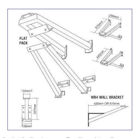
CCTV systems require quality engineering support - and that is exactly what the Shawley range offers. Heavy duty wall or corner mount brackets and tripods are manufactured from the mild steel box tubing and powder coated for long life protection. They provide the perfect support for pan and tilt heads, housings and infra-red illuminators.
