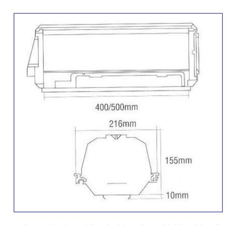
Shawley's extruded aluminium housings have been designed with an eye for aesthetics, whilst the hinged sunshield and hood allows complete access to camera and lens assembly. The central body is manufactured in extruded anodised aluminium with die-cast aluminium end caps finished with black polyester.
