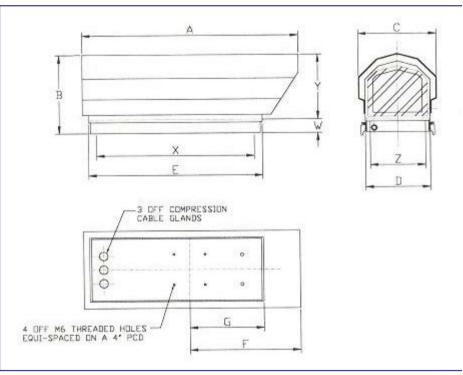
The CH9, CH10 and CH11 camera housings have been designed to supplement the CH range with a stylish alternative. Manufactured to the same high standards of all Shawley equipment, they come complete with IP66 rating, demister/heater, compression glands, laminated glass, sunshield and adjustable camera platform. The units are built as 240vAC standard, but other voltages are available on request. As with all the CH range of housings, integral wipers can be fitted.
