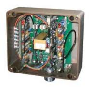
Each FPS-5 processor validates the communication packet before re-transmitting the information to the next processor. The FPS-5 audio signal is digitized and interleaved with the data packets on the same fiber optic cable. This technique eliminates the need for a dedicated audio BUS.
