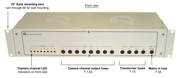
\*The 8 LED indicators on the front panel provide verification that power is on to the camera channels. If an LED is not lit then power has been cut to the relevent channel. The most likely cause of this is a blown fuse. Fuses are located on the front panel.
