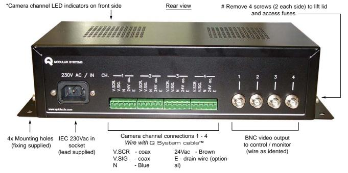
\*The 4 LED indicators on the front panel provide verification that power is on to the camera channels. If an LED is not lit then power has been cut to the relevent channel (read from <u>right to left</u> 1-4) The most likely cause of this is a blown fuse. Fuses are located within the unit as shown below. # Remove lid to access
