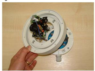
3. Disconnect the camera connector from the power board. Remove the 4 off M6 screws & seals retaining the body ring to the ☐ Socket™ and separate the body ring from the socket as shown.
