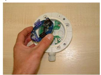
4. Remove the 2 screws, lift away & disconnect the power board from the socket. Follow the supplied ☐ Socket™ instructions for mounting and wiring of the socket. Re-assemble ☐ ToughEYE™ in reverse order to finish.
