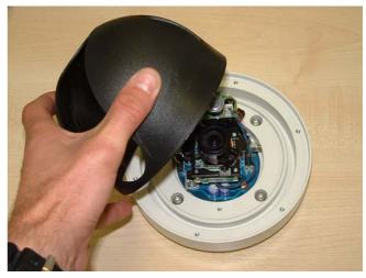
2. Lift the inner hemisphere from the body. The inner hemisphere is friction retained and requires no tools.
