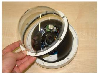
1. Unscrew the 6 off fixings retaining the outer polycarbonate hemisphere and remove. *Take care not to scratch the material.*
