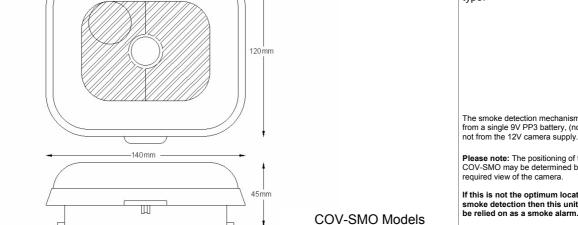
The smoke detection mechanism operates from a single 9V PP3 battery, (not included)
