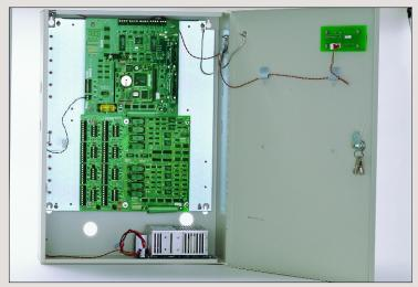
PCSC retains its leading role in intelligent controllers products by offering the Ultimate™ Series, a 100% distributed architecture with open architecture to support TCP/IP protocols and direct connections to LAN/WAN networks. It offers superb management of access control, alarm monitoring and output control subsystems.
