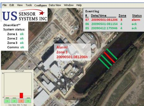
typical DiverAlert™ system display. In addition to a map view showing the alarmed zone and a pop-up box providing information about the alarm, a signal strength bar chart is also provided, with the signal strength of each of the sensors displayed concurrently. An event log provides historical information about the most recent alarmed events. The system constantly monitors all of the zones as well as the communications link to alert the user of any system level problems.
