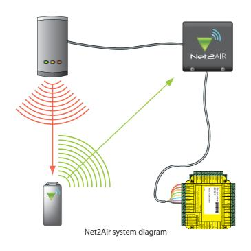
A Net2Air hands free interface is simply installed between the PROXIMITY P series reader and the Net2 access control unit.
