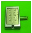
memory and intelligence inside the body of the keypad. The benefit of this is that installation wiring is very simple. **TOUCHLOCK compact** is the membrane version. It has three twin core cables coming out of the rear of the keypad. The black cable connects to a 12 volt power supply and the white cable connects to the lock. A
