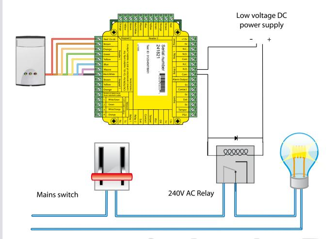
The Switch2 controller can be used for the same function. Set the unit to operate in toggle mode with a function card. The mains relay is again wired across the COM/NO/NC Switch2 terminals as required.
