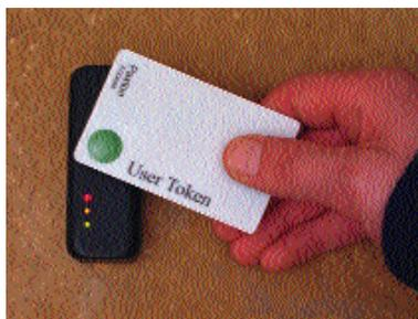
PROXIMITY provides all of the convenience of proximity reading technology combined with the same ease of use and system management as CARDLOCK.
