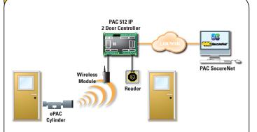
The Wireless Module offers the ability to seamlessly connect the ePAC Cylinder to PAC controllers and provides the following benefits:
