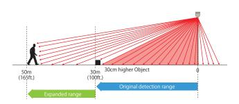
Within 30m radius (100 ft.) range, the unit can detect a moving target with a minimum width of a 30cm (1ft.). Within the extended detection range between 30m and 50m range (100 ft. to 165ft), the RLS-3060Sh can detect objects which are at least 60cm (2ft) wide with 10% reflectivity. The extended detection area can be used to detect larger objects such as vehicles and forklifts but not people.
