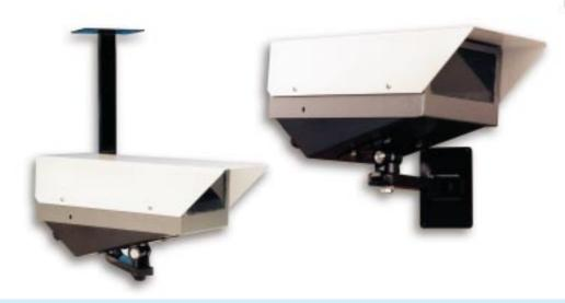
Available in 24vAC or 240vAC versions, the Surveyor camera housing incorporates a panning camera platform enclosed within a heated environmental housing designed to IP65 standard. The unit will accommodate most compact CCD cameras with fixed lenses. With the adjustable camera sweep a standard fixed I/2" 6mm lens will give a panning field of view of approximately 88°, ideal for garage forecourts, loading bays, yards, car parks etc.
