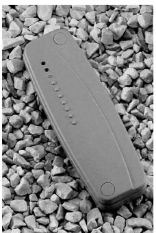
**exchange**. Visual indication of reader state is established by means of 3 LED's and an internal sounder is provided for audible confirmation of card read. The fully encapsulated electronics are housed in a tough, all weather ABS case with front fixing points. Fixing screws and blanking plugs are provided.
