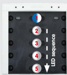
Pattern 1 (MX-Bell-Button-F1): LED 1 permanently blue (function button) LEDs 2 to 5 flashing white (bell buttons)
