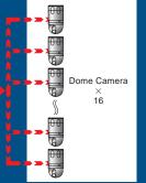
Up to 16 dome cameras can be connected with the machine. Even different manufacturers' dome cameras can be mixed and controlled individually using an remote controller.
