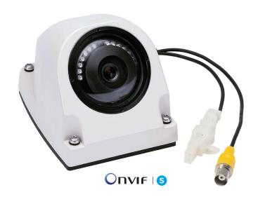
The **Mobile IR Wedge Camera** from March Networks® provides flexible mounting options — both interior and exterior — for vehicles deploying cameras. The ruggedized housing protects the camera from dust and moisture, and its vandal-resistant aluminum design, with polycarbonate dome cover, is built to withstand the harsh transit environment of bus and rail vehicles, including wide temperature swings and humidity.
