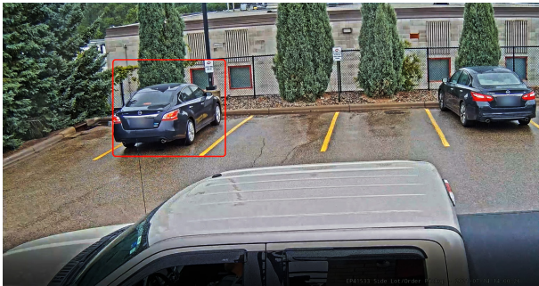
The "Stopped Vehicle" analytic triggers an alert when a vehicle pulls into a parking space for curbside pickup.
