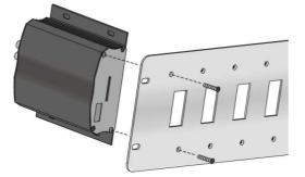
**3.** Please connect 12 VDC connectors into the Video Codecs. After all the devices are properly installed, install the Rack Mount Plate on the rack using the four mounting holes.
