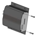
2. Install the device on the Rack Mount Plate with the supplied screws of the Video Codec as in the following way:
