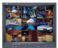
provided. Cameras, channels, and split pattern can all be specified without using a splitter. Images can be displayed on a single screen or on split screens (4, 6 and 9).
