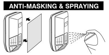
The anti-masking & spraying system detects the unit being masked or sprayed (approximately 30cm for 10 sec.). The trouble LED will flash to indicate this condition. Trouble output format can be selected by the repositioning of the DIP switch PIN 6. The anti-masking function is activated by the removal of jumper loop JP7. (Only available on IR-150AM & IR-150QA)
