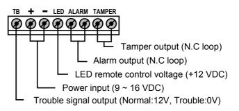
TAMPER terminals to be connected to a 24 hours N.C supervisory loop of control panel.
