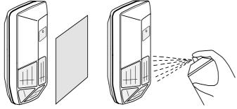
The anti-masking & anti-spraying system detects the unit being masked or sprayed (masking approximately 25cm or sprayed after 10 seconds). The alarm LED will latch and a trouble signal is transmitted to the control panel through "TB" output terminal. The trouble output format is selected by the "A-M." PIN 6 switch.
