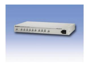
The MVF-60/ 90 series Multiplexers have a feature of monitoring the six (MVF-60) and nine (MVF-90) camera picture, display Quad (A/B), Six (MVF-60) and Nine (MVF-90) split views, video output to VCR while sequentially switching the pictures from cameras, as well as monitoring of desired channel picture selected from the recorded video data in VCR's or DVR's.
